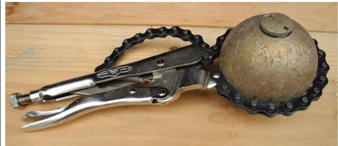
A strap wrench is useful with softer metal implements or where leaving scratches is not desired. The strap should be 18" long to fit 130 mm shots or hammers.
