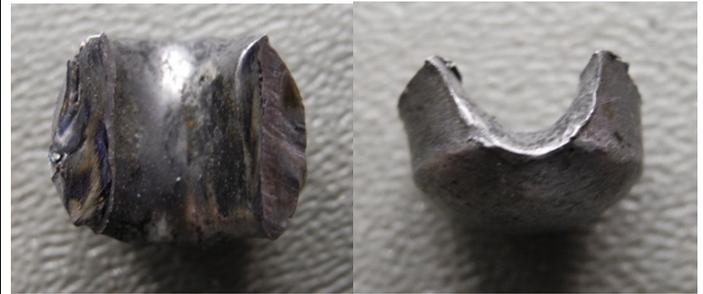
Time permitting, it's a good idea to look at the hammer lugs for hairline cracks or necking of the material. Such conditions will lead to failure of the lug during a throw.
